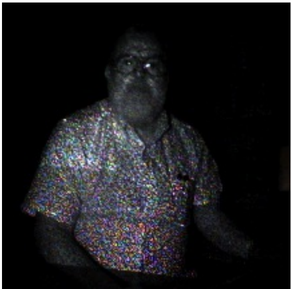
Figure 1. What the Kinect IR camera sees
