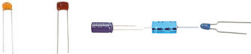
Figure 6. Capacitors: Ceramic, mylar, radial electrolytic, axial electrolytic, tantalum.
