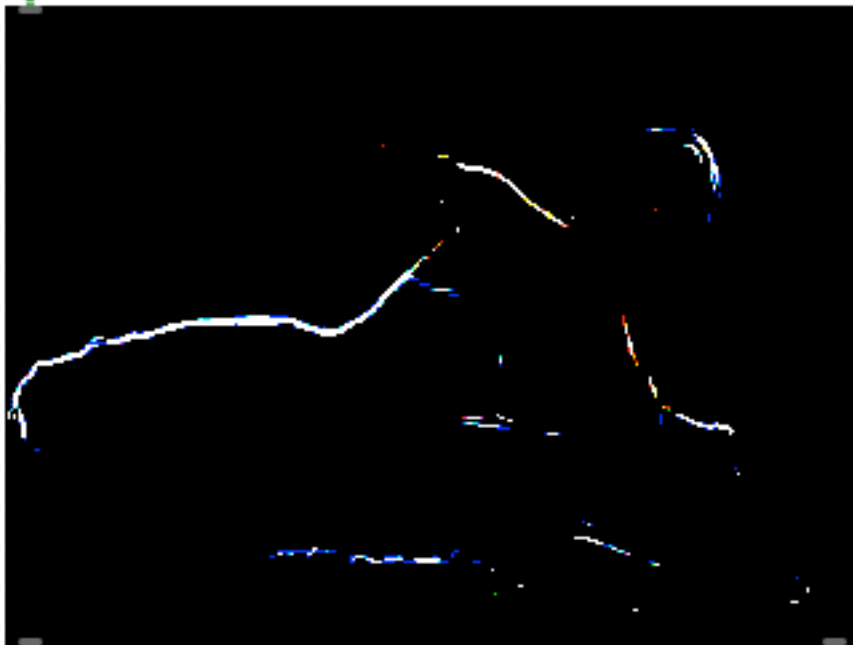
Figure 10. The jit.op > sets pixels above a threshold to 1. This removes the faintest details and brightens what remains. The process works plane by plane, so some pixels are blue or red. This image is suitable for the feedback smear shown in figure 4.
