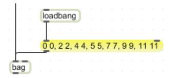
The gotcha with loadbang is that if you have several, you won't know which will bang first. The answer to that is to have only one attached to **send** objects that distribute the bang in a controlled order. **Loadmess** is a new version that will send more than a bang.
