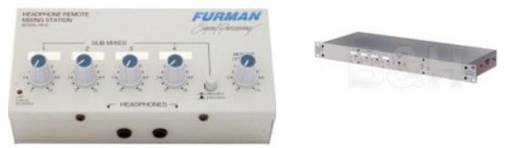
The Furman system provides individualized headphone mixes in the studio. There are four headphone stations permanently mounted in the studio. These receive six signals, and the mix is adjusted by controls on the box. The right hand knob controls the main mix, and the four extra knobs bring in extra signals chosen at the console.
