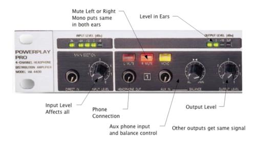
There are four output sections- note that there is a headpone out and Aux in jack on each section. It's easy to get them mixed up, but you will not hear anything from phones connected to Aux In. In addition to the front jacks, three of these sections feed remote jacks.
