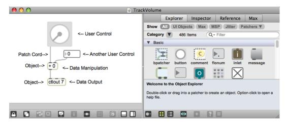
The sidebar can show an object explorer, the inspector for a selected object, the reference page for a selected object, or the Max window.
