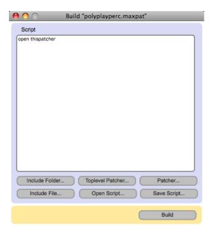
Finally, the build button lets you name and save the collective. A collective should run under either version of runtime, Mac or PC.
