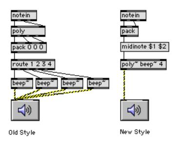
Note that the logic of selecting which instance of beep~ is playing a particular note is a bit different in the two. The problem of course, is getting the note off to the proper beep~.
