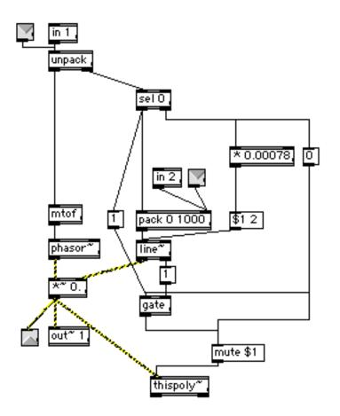
When the note on comes in, the mute 0 happens unequivocally. We need to get the mute 1 from the bang at the end of line~, but this also bangs on the way up, so it has to be prevented by a gate until it's really needed. The right outlet of this poly~ shows the mute status, so its easy to test.
