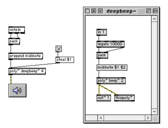
The deepbeep~ patcher depends on the legato object (that's an Lobject) for the switching logic. Legato will provide a note off message for the playing note just before sending the new note. (Legato is a version of makenote. There's a duration parameter, which is set to 10 seconds in this example.)
