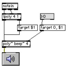
Here, I'm using the lpoly<sup>1</sup> object to manage the polyphony of poly~. In this configuration, the voice number chooses the target before the note message arrives. Lpoly uses a ripoff algorithm I prefer to the one in poly~<sup>2</sup>. You can easily roll your own in a patcher object. The right inlet controls the decay time of the beep~ patcher. (see page 3) The target 0 preface sets all instances to receive the message.
