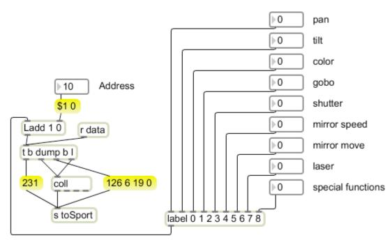
Figure 3. The number boxes routed through Label generate the messages for each parameter of a lighting instrument. The Ladd will offset these to the starting address for each instrument.
