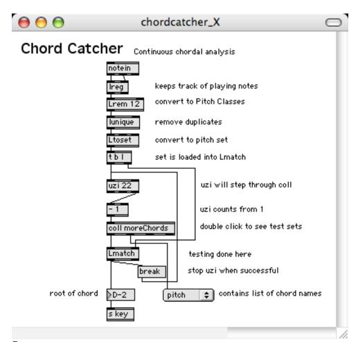
Figure 7. For details of how this works and the contents of the moreChords coll, see the essay <u>Max</u> & Chords.
