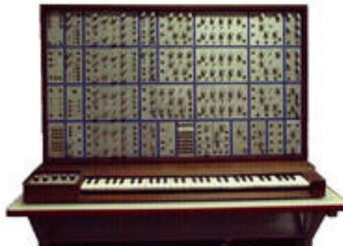
An analog synthesizer is a collection of electronic circuits that are useful for generating and manipulating signals that will ultimately be heard as sound. In the classic MODULAR SYNTHESIZER each circuit is separate and interconnections are left up to the user. In the PERFORMANCE SYNTHESIZER the circuits are already interconnected in a pattern the manufacturer thinks is most likely to sell. This discussion is going to deal with modular synthesizers.
