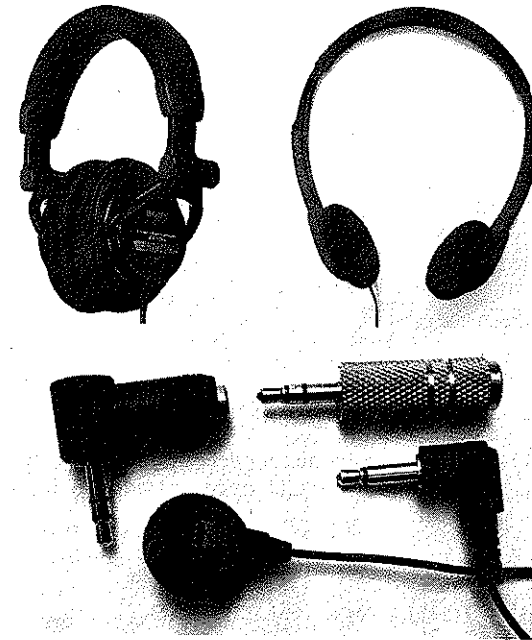
Fig. 11-2. (upper left) Headphones with closed earpads. (upper right) Headphones with open earpads. (bottom) Mono earpiece shown with mono connector; stereo-to-mono adapter (so you can hear both channels from the camcorder); and right-angle adaptor (so the plug doesn't stick out from the camcorder).
